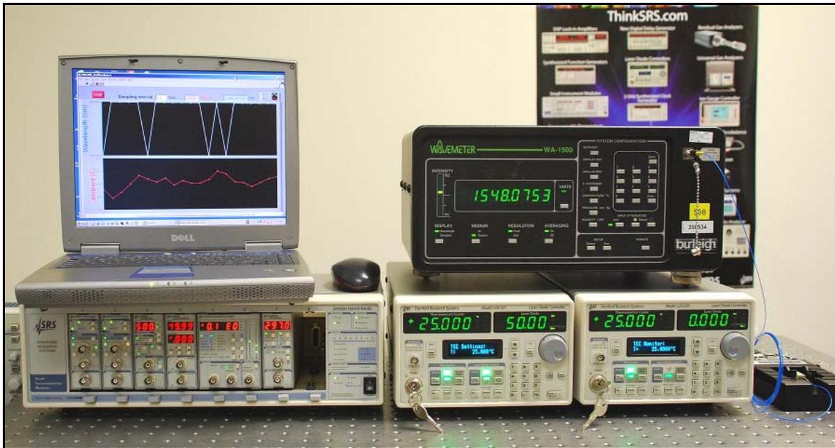
**Figure 1** Wavelength drift test setup
