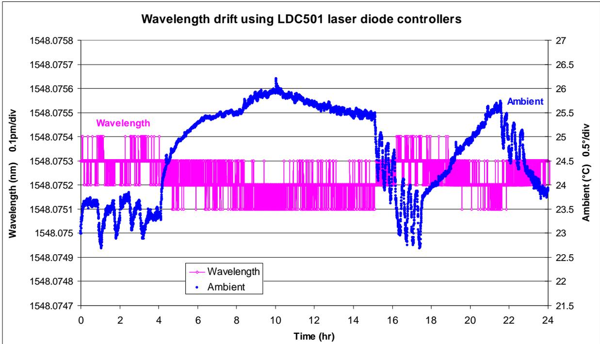
**Figure 2 Overnight wavelength drift of a butterfly laser controlled with a LDC501**
